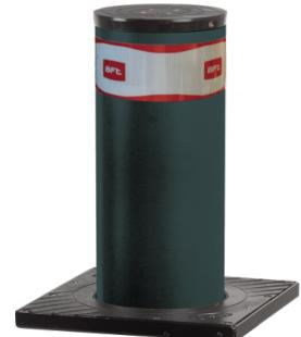
Anti-terrorist hydraulic bollard with incorporated hydraulic control unit. Suitable for protecting sensitive sites, thanks to the special "SD" version, which keeps the shaft raised in case of a power failure and with public installations where, in the standard version, the shaft lowers automatically with no power.
